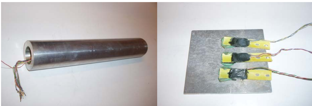
Figure 4.17 Aluminium cylinder with attached strain gauge rosettes to the left and aluminium slab with strain gauge rosettes to the right.
